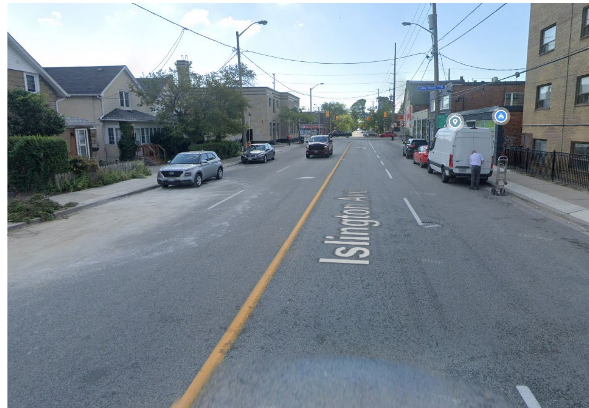
Islington Avenue Four traffic lanes, off-peak parking in curb lane on both sides
