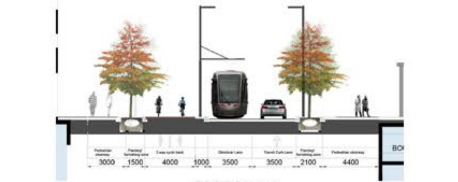
SECTION A-A LOOP ROAD - 23.0m R.O.W.
