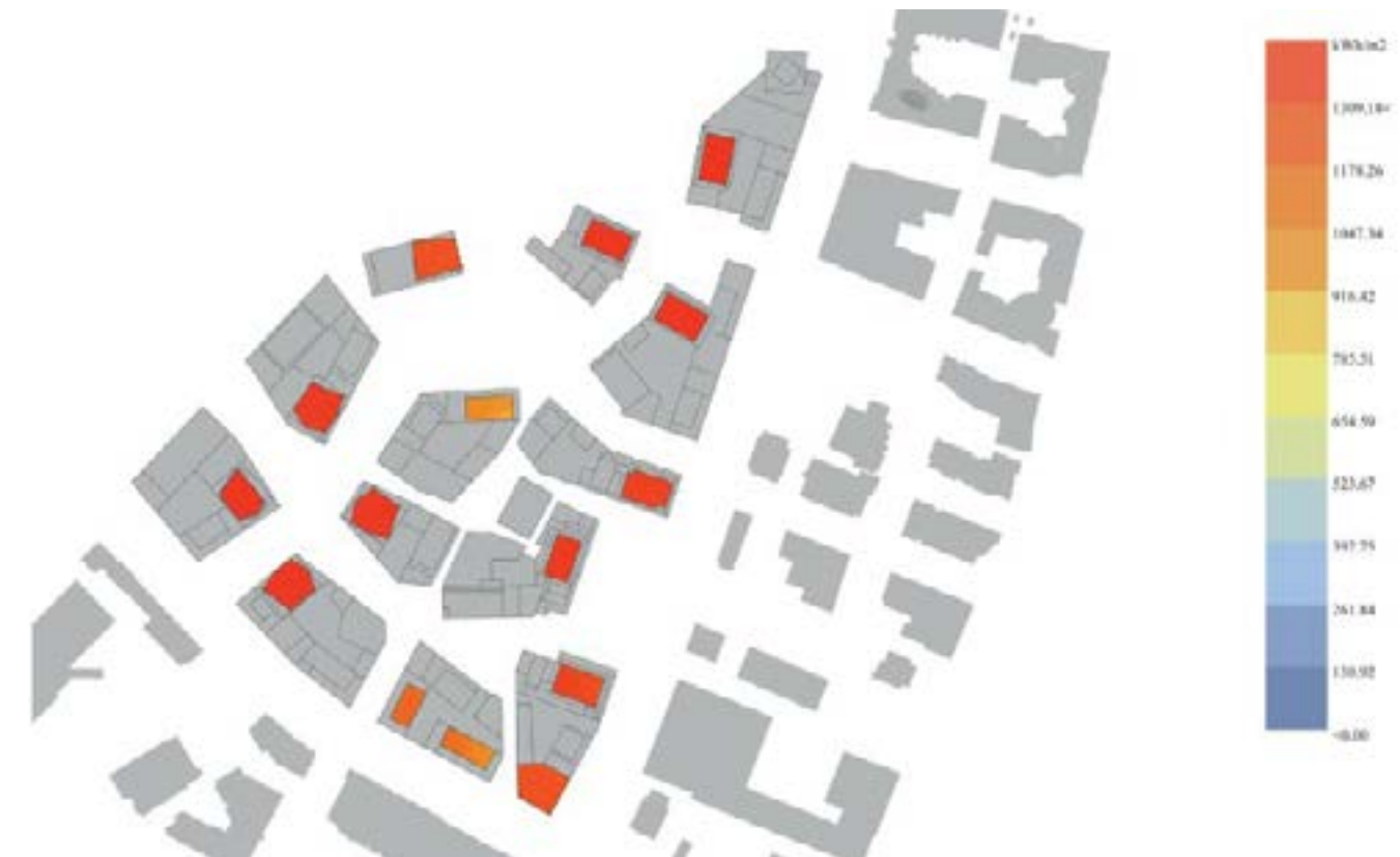
Figure 16 - Solar panel location and solar radiation in Scenario 2 - Plan view.
